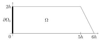
The above problem is discretized using *linear finite elements* with the following triangulation:
